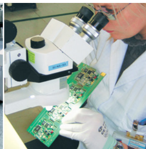
Visual inspection station
